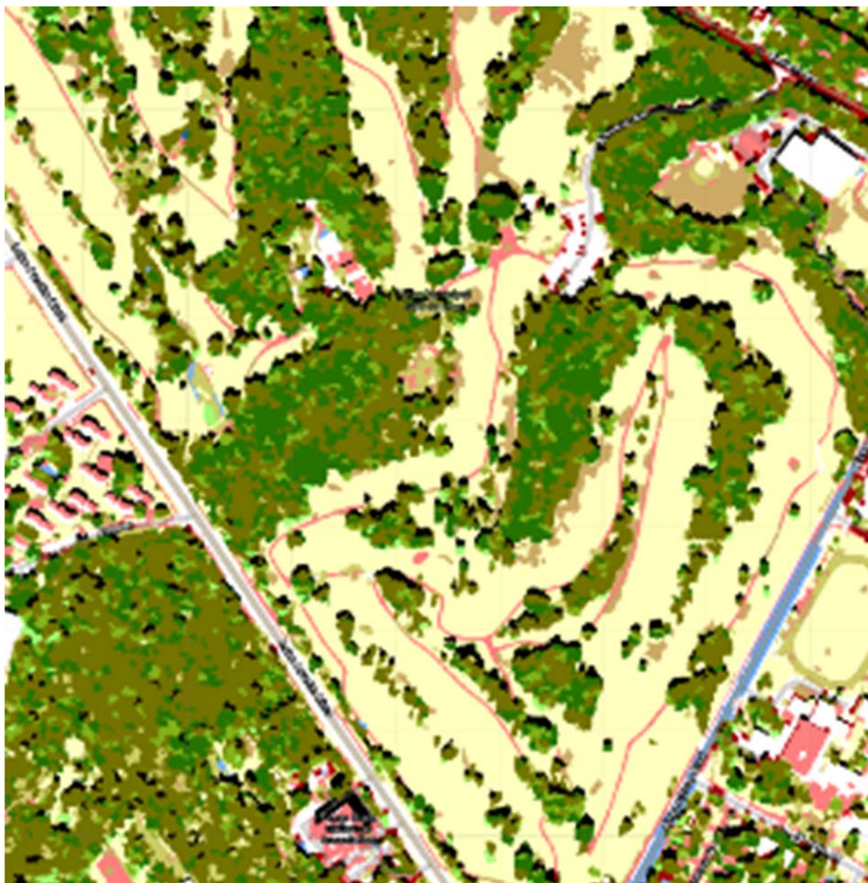
Figure 6-4. Landcover map (50 cm resolution) of Lions Municipal Golf Course in Austin showing trees (various types in different shades of green), grass (yellow) and bare soil (brown), buildings and pavement (white, grey and red).
