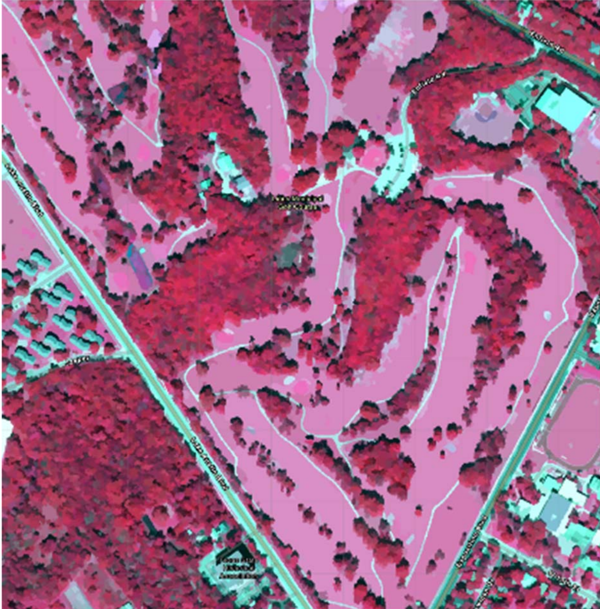
Figure 6-3. Object based segmented image based on 50 cm NAIP visible and IR bands. The figure shows the Lions Municipal Golf Course in Austin TX. Trees are dark red, grass is pink, buildings, roads and trails are grey/bluish/white in this false color image.
